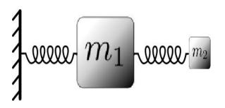
Considering this as a classical system, we expect that the motion will be dominated by the large heavy particle (m1), which is attached to a fixed wall by a spring. The small, light particle (m2), which is attached to the heavy particle by a spring will simply follow the heavy particle and execute rapid oscillations around it.
