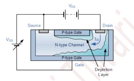
The FET however, uses the voltage that is applied to their input terminal, called the Gate to control the current flowing through them resulting in the output current being proportional to the input voltage. As their operation relies on an electric field (hence the name field effect) generated by the input Gate voltage, this then makes the Field Effect Transistor a "VOLTAGE" operated device.
