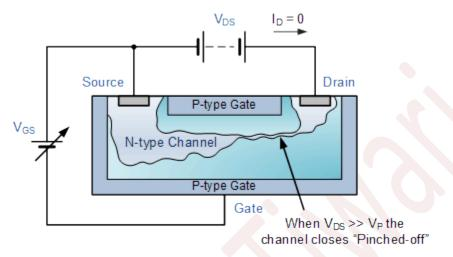
In this pinch-off region the Gate voltage,  $V_{GS}$  controls the channel current and  $V_{DS}$  has little or no effect.
