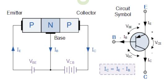
(Note: Arrow defines the emitter and conventional current flow, "in" for a PNP transistor.)
