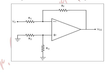
You can observe that the voltage at the non-inverting input terminal of the op-amp will be zero volts. It means, the above circuit is simply an inverting op-amp. Therefore, the output voltage  $V_{02}$  of above circuit will be –
