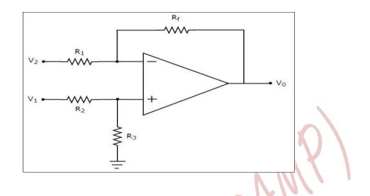
Now, let us find the expression for output voltage  $V_0$  of the above circuit using superposition theorem using the following steps –
