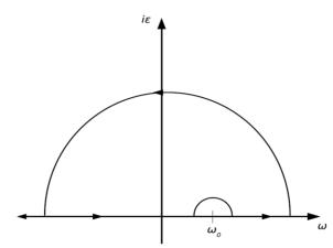
Fig.1 Contour in the complex frequency plane
