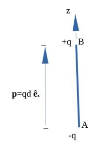
Now, if we somehow change the charges at point A and B with time. Moreover, if the change is such that charges at point A and B become the oscillatory function of time i.e., for example:
