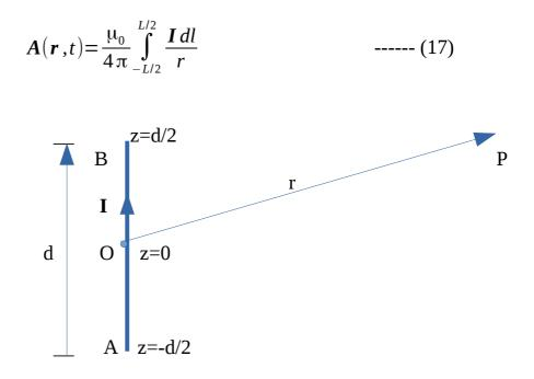
We can treat the oscillating dipole as a current carrying wire of length d oriented along z-axis such that the center O of the dipole is located at the origin z=0. Then the coordinate of one end A of wire is z=-d/2 and the coordinate of another end B is z=-d/2 (see above figure). And we can consider length element dl = dz. The current passing through the dipole is given by equation (16). Using all these inputs in equation (17) to calculate the retarded vector potential associate with the dipole,
