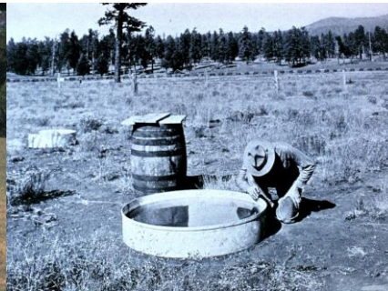
From U. S. Forest Service GAGING THE THIRST OF THE AIR The observer is measuring the depth of water in the evaporation pan with a graduated glass tube (burette)
