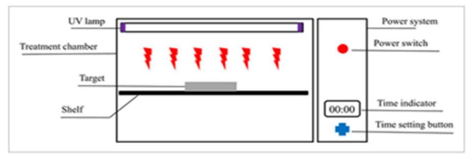
Fig: Diagram of a pulsed UV light system for treating food stuff (From - Google)
